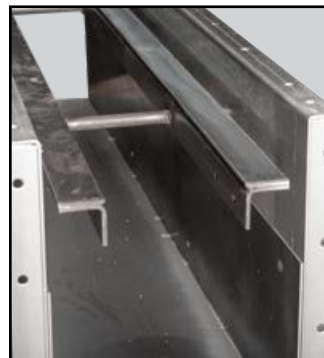
Chain return rails are capped with 1/4-inch (6.4-mm) AR steel for longer life.
